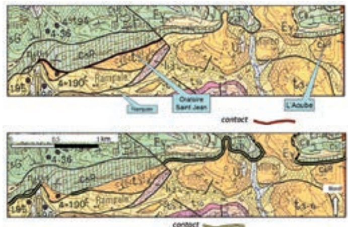
Figure 3. a: The "transgressive" contact between Santonian CsR and Trias t3-6. b: The tectonic contact between Santonian CsR and Trias t3-6.
